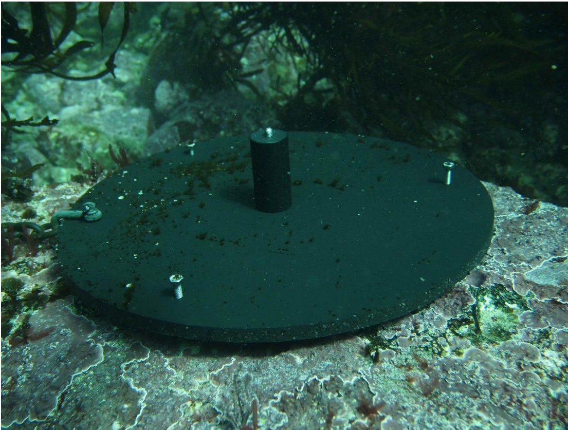
Figure 3. ARM with HDPE locking nut and three riser bolts on the perimeter. Lighter chain tether securing the plate to the main locating chain can be seen on the left.
